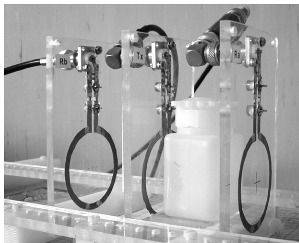
Fig. 1. Prototype of the RF system made of three parallel circular loop RF surface coils. The center-to-center distance ( d_{cc} ) between each pair of RF coils was 6.0 cm. Each coil (diameter 5.5 cm) was built on a Plexiglas substrate and was made of adhesive copper tape (width 5 mm, thickness 150 \mu\text{m} ). A trimmer capacitor (1–16 pF) was connected for tuning the RF coil at f_0 = 100.00 \pm 0.01 \text{ MHz} when isolated. A capacitive balanced network was used for impedance matching [19]. A BNC coaxial connector was mounted on the Plexiglas substrate and used for connecting the coil to the RX via a 50 \Omega coaxial cable (RG58). The measured quality factor Q was 132 when empty and it decreased to 110 in the presence of a phantom containing 500 ml of physiological saline solution.
